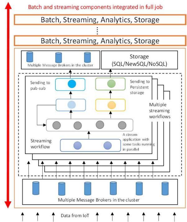
Figure 4. Apache Storm processing data from Internet of Things (IoT)
